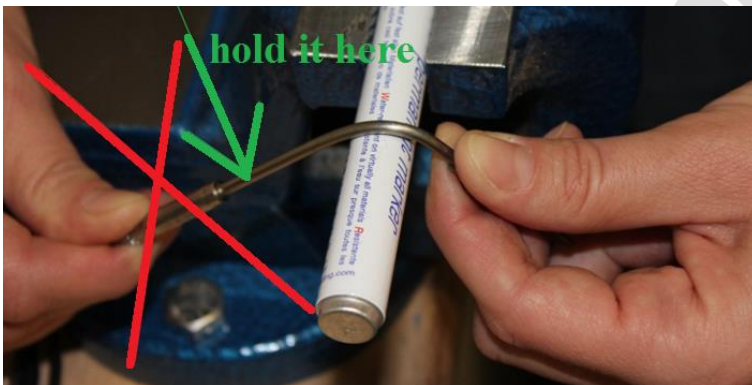
Fig.: Bending the thermocouple over a circular shape. Never press the transition sleeve.
